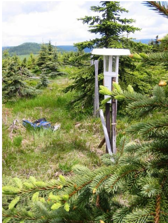
Installing fog collector (photo: Josef Krecek, 2010)
