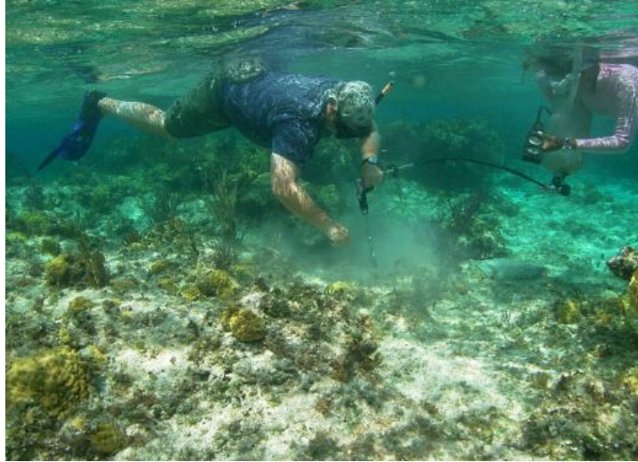
Photo 3. PI John Rollino and project Staff Scientist Ms. Anne Paul, use a pneumatic drill to secure a RED to the reef.
