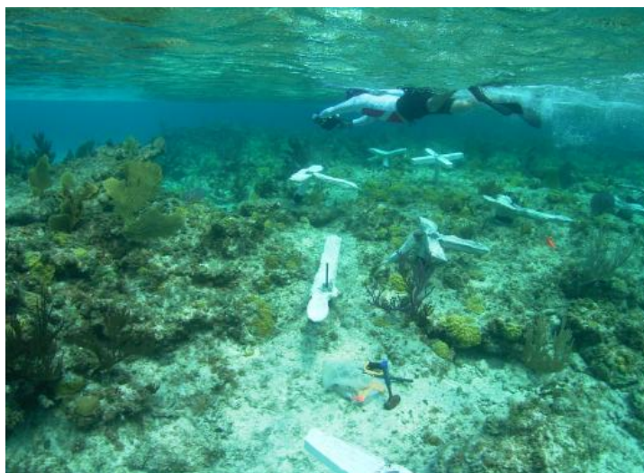
Photo 1. Rugosity Enhancing Devices placed on the Reef
