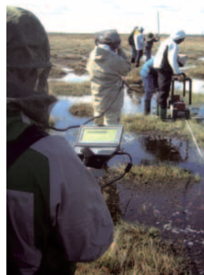
Volunteers conduct ground-penetrating radar surveys along transects to measure permafrost thickness.
