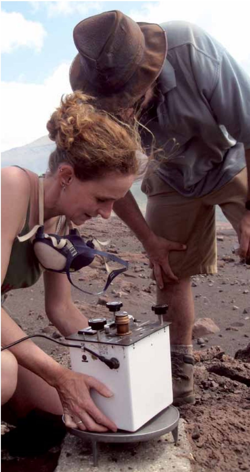
Figure 2: Teams use gravity meters to study micro changes in gravity caused by movement of magma within the volcano.
