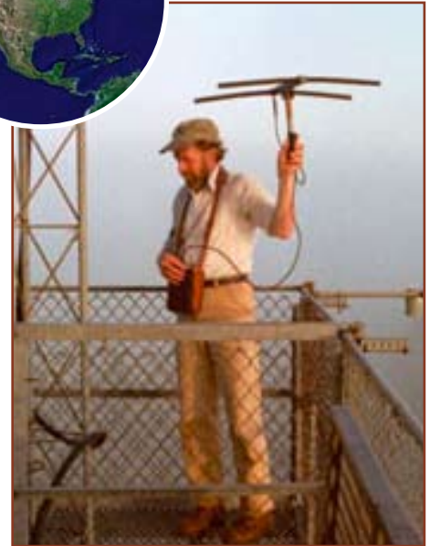
Scientist using radio telemetry to locate animals. This antenna picks up a signal transmitted from collars around an animal's neck.
